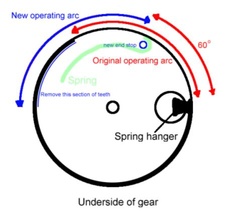
Note the thickness of the edge of the gear. There is a thin section where the end stop screw runs. It goes from the point where the spring hooks on, to a point approximately 120 degrees further round. This thin area has to be extended by 60 degrees. Clamp the gear in a vice and remove a section with a hacksaw, then clean up the edge with a file.
