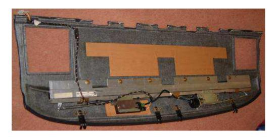
Unplug the motor from the control unit. Cut through any cable ties securing the wire to the shelf. At the far end of each arm, pry off the one-way washer holding it to the actuating arm. Mark the position of the 3 screws on the rear of the motor mounting plate and remove the screws. The gearbox can be removed from the shelf with the arms still connected, the longer one has to be carefully threaded out.
