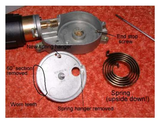
Put a bit of grease on the spring and replace it back behind the gear, in the same orientation as it came out (shown in the diagram in green). NB it is upside down in the picture, with respect to the orientation of the gear. The diagram is correct. Put a bit more grease around the teeth of the gear, align it with the gearbox and replace it, remember the centre of the spring has to line up with the centre spring hanger.
