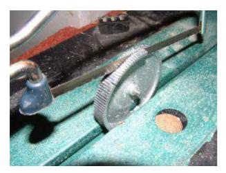
The point where the spring hooks on also has to be moved 60 degrees round the gear, and the old mounting hook has to be removed. I removed it with a cutting bit in my mini drill. The new mounting point can be created by drilling and tapping a small hole in the gear, then driving a machine screw through the hole to form a peg for the spring. Remember, this peg is also the end stop, and you will probably find that the end stop screw in the gearbox casing is
