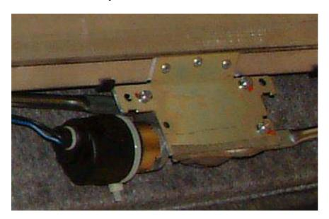
Turn the motor over and unscrew the centre screw from the actuating arm wheel. Pry off the wheel. Before you attempt to unscrew the gearbox, beware. There is quite a powerful spring behind the main gear, to assist it in raising the blind. The tension in the spring needs to be relieved before the gear can be removed. For absolute safety this can be done before you unscrew the gearbox, although with a little care it is possible to do it after opening the gearbox.
