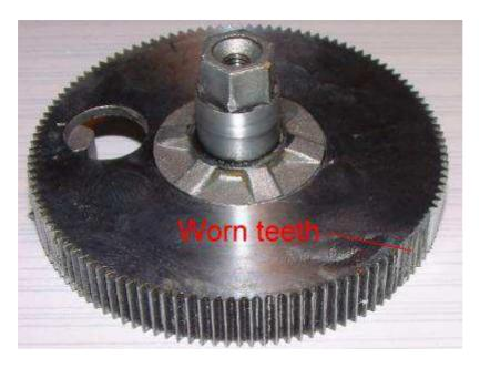
Note the output shaft of the gear. It has a hex end on it, so each face is at a 60 degree angle to the next. Because we want the output wheel to start and end in the same relative position as before, we need to use a section of gear which is a multiple of 60 degrees away from the section it was originally using. See diagram.
