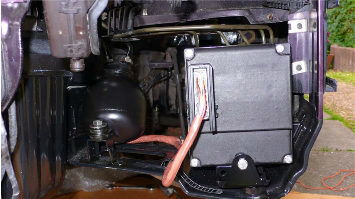
Picture-22: Clean, lubricate and refit the main wiring connector.
