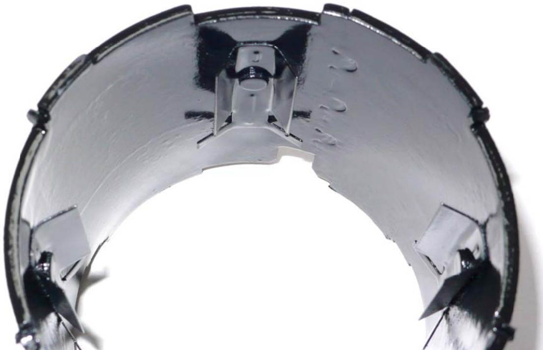
Picture-16: Clean and paint the inside of the stator tube (note the clips which retain the magnets).
