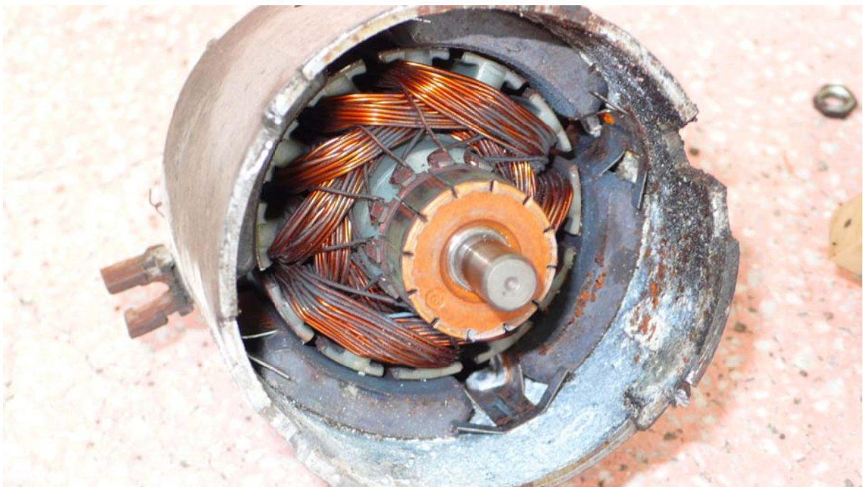
Picture-10: Motor commutator and windings could do with a clean. Note ceramic magnets are held in by spring-clips
