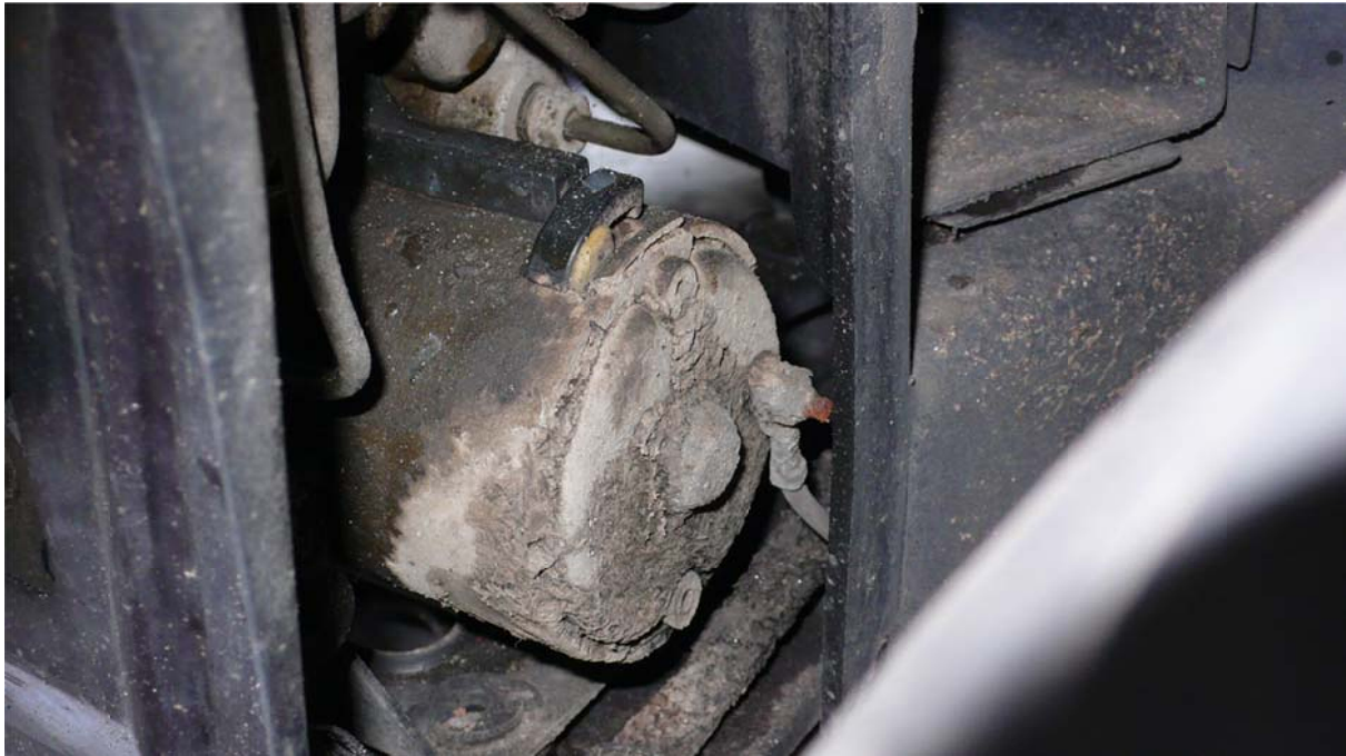
Picture-1: Before Cleaning. (The wheel arch liner does not offer good enough protection and the unit is also exposed to water and dirt from above, from the headlight openings.)
