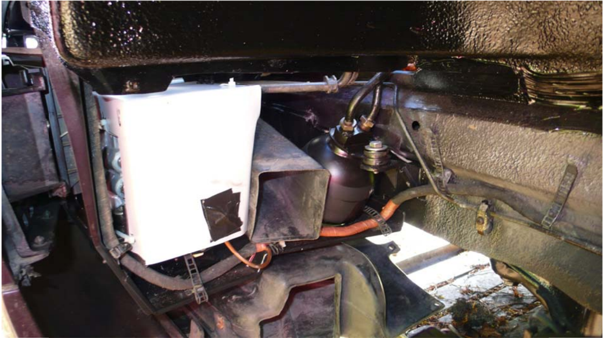
Picture-24: The cover extends down to the rear.
