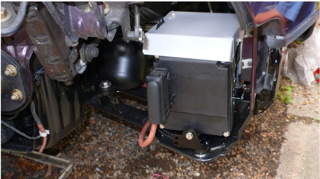
Picture-23: A cover made of thin sheet zinc is added to protect the ABS unit from rain and dirt. The cover is secured to the hydraulic lines on one side and to the chassis on the other using cable-ties.
