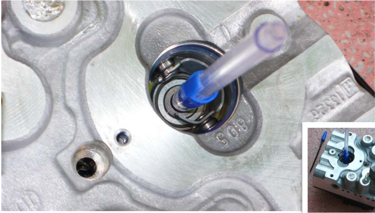
Picture-13: using some WD-40 and the end of a Bic biro to rotate it, it was freed-up and some Isopropyl alcohol was then used to clean it.
